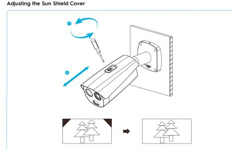
Loosen the adjusting screw on the base of the camera to adjust the device. Once finished, tighten the adjusting screw firmly to lock it into position. Do not rotate the device over 360° when the
